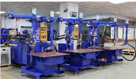
Applications of Dual-Gun Platform-Type Spot Welding Machines in Sheet Metal Fabrication Plants
