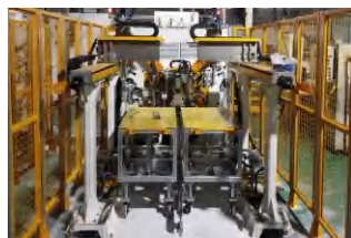
Four-Point Welding Machine for Automobile Shock Absorber Connecting Rods
