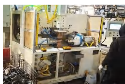
Double-Sided Spot Welding Machine for Automotive Brackets
