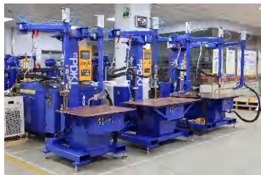
Back-Side Indentation-Free Copper Platen Spot Welder (Single welding gun)
