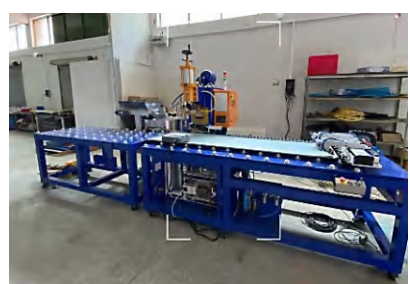
Dedicated Automatic Projection Welding Machine for Door Panel Hinges
