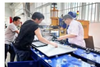
Dedicated Automatic Projection Welding Machine for Door Panel Hinges
