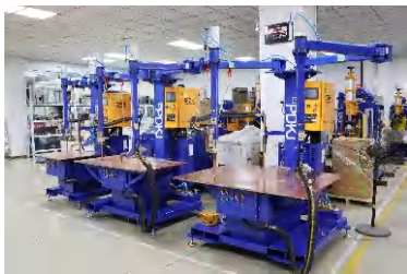
Back-Side Indentation-Free Copper Platen Spot Welder (Dual welding gun)
