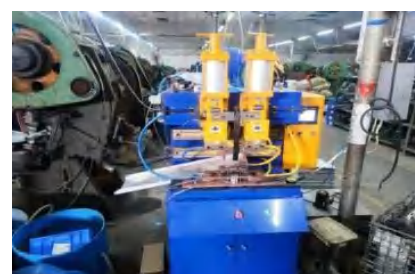
Automatic Spot Welding Machine for U-shaped Clips on Door Panel Reinforcements
