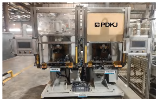
Double-Sided Projection Welding Machine for Automotive Shock Absorber Brackets
