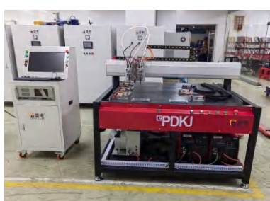
CNC-Controlled Triple-Gun Automatic Stud Welder
