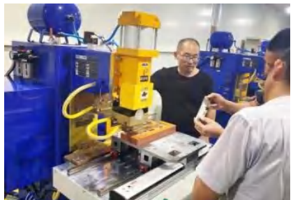
Automatic Spot Welding Machine for MOSFET Spring Clips
