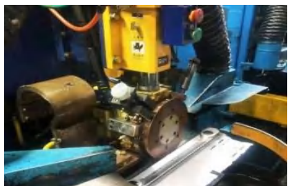
Circumferential Welding Machine for Oil Radiator Heater Fins
