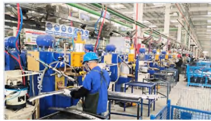
Welding Applications of Stationary Spot Welding Machines in Automotive Manufacturing Plants
