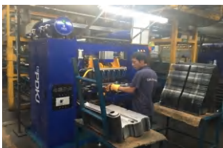
Automatic Multi-Spot Welding Machine for Oil Radiator Heater Fins
