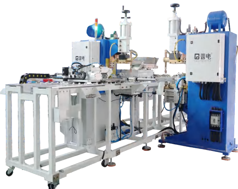
Automated projection welding machine for automotive door panel hinges
