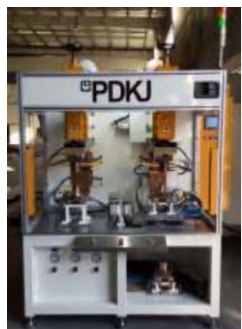
Dual-Head Projection Welding Machine for Automotive Subframes
