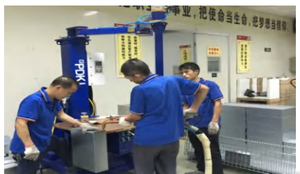
Application site of the traceless spot welding machine on the platform
