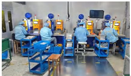
Precision Spot Welding Machines Utilized in Electronic Manufacturing Plants
