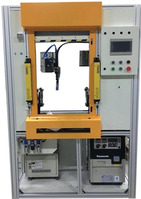
Automatic welding equipment for automotive steering gears
