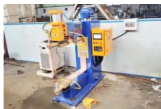
Dedicated Medium-Frequency Welding System for Extended/Heightened Telecom Cabinets
