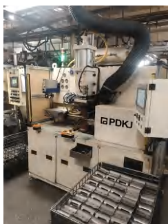
Double-Sided Projection Welding Machine for Automotive Shock Absorber Brackets
