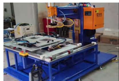
Automatic XY-Axis Spot Welding Machine for Computer Cases
