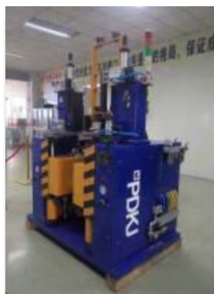
Circumferential Welding Machine for Oil Radiator Heater Fins
