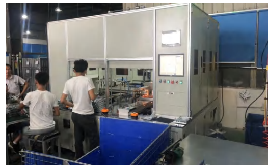
Dual-Station Automatic Welding Workstation for Computer Cases
