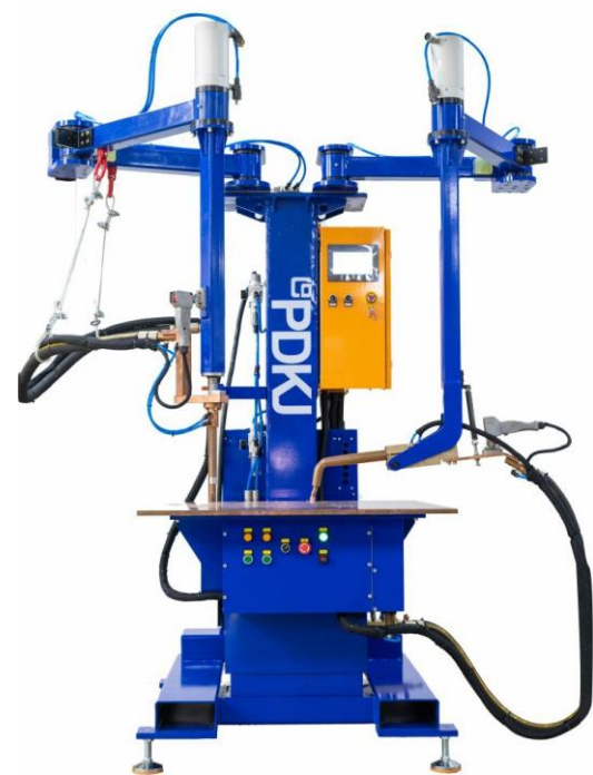
Double - gun platform type medium frequency inverter spot welding machine
